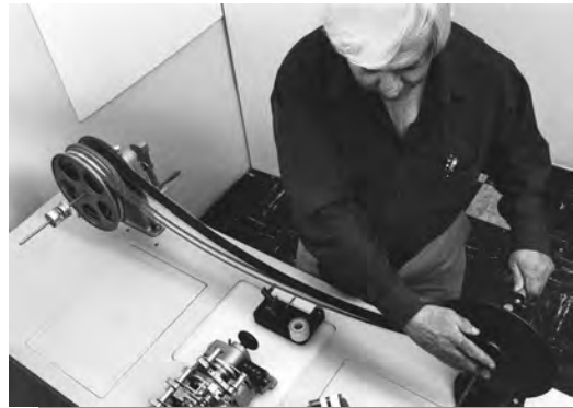
S.u. Flanging Moviola roll from coded daily reels.
