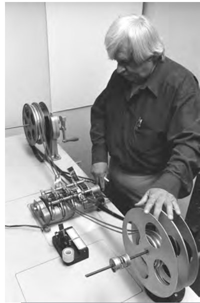
S.s. Syncing dailies: preparing to grease-pencil the track in two gangs. Spring clamp is at end of rewind in foreground.
