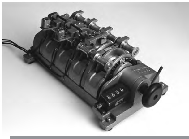
5.a. Synchronizer zeroed out; two sound heads up, one down.
