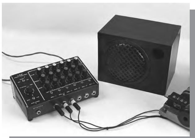
S.d. Modern squawk box and speaker with synchronizer.
